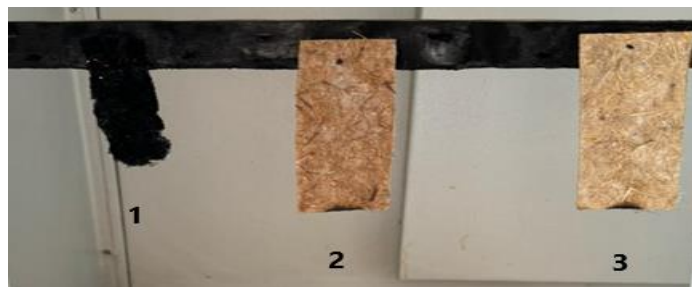
1- untreated sample; 2- a sample treated with a compound of guanidine hydrochloride and sodium phosphate; 3- sample treated with Nortex-KP
